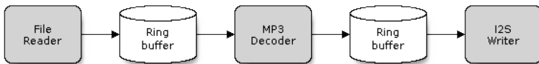
Fig. 2.4: Ring Buffer used in Audio Pipeline
